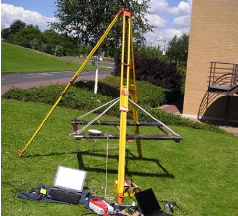
Figure 4 Platform for a Dynamic Test Using JNS100 and Leica receivers
