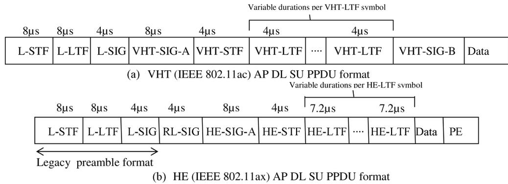
**Figure 2.** The PPDU format in single user (SU) mode in IEEE 802.11ac and IEEE 802.11ax.
