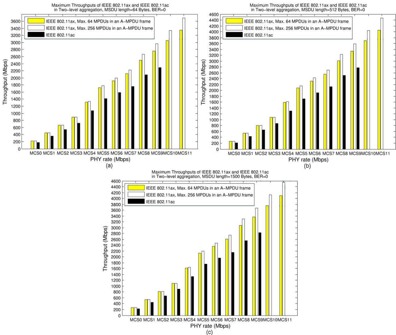
**Figure 3.** Comparison between the maximum throughputs of IEEE 802.11ax and IEEE 802.11ac in the two-level aggregation scheme, single user operation mode.  $BER = 0$ .
