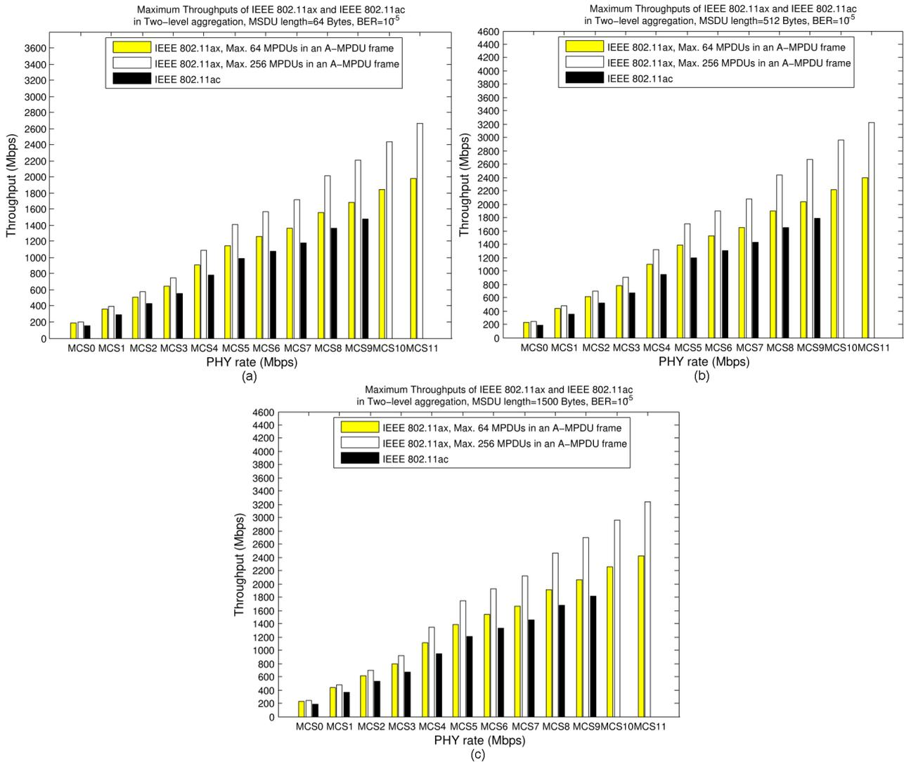
**Figure 4.** Comparison between the maximum throughputs of IEEE 802.11ax and IEEE 802.11ac in the two-level aggregation scheme, single user operation mode.  $BER = 10^{-5}$ .
