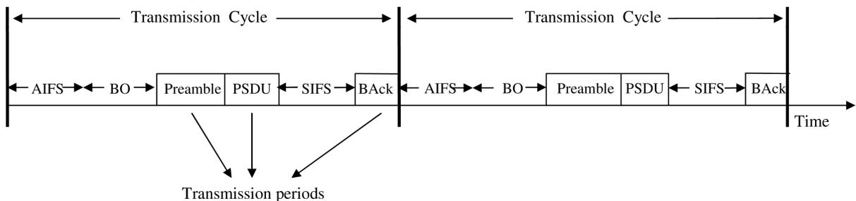
**Figure 1.** Transmissions from the AP to stations in single user mode in IEEE 802.11ac and in IEEE 802.11ax.
