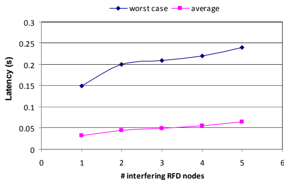
Figure 13. Transmission latency vs. # RFD interfering nodes (10 RFD transmitters).
