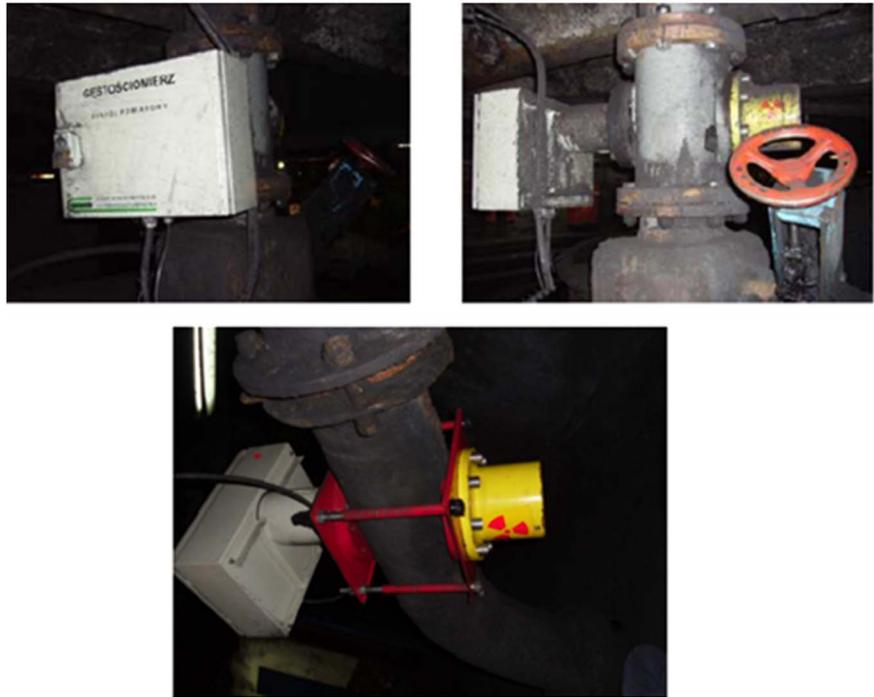
**Figure 5.** Density gauges into coal enrichment installation (source Cs-137) [13].
