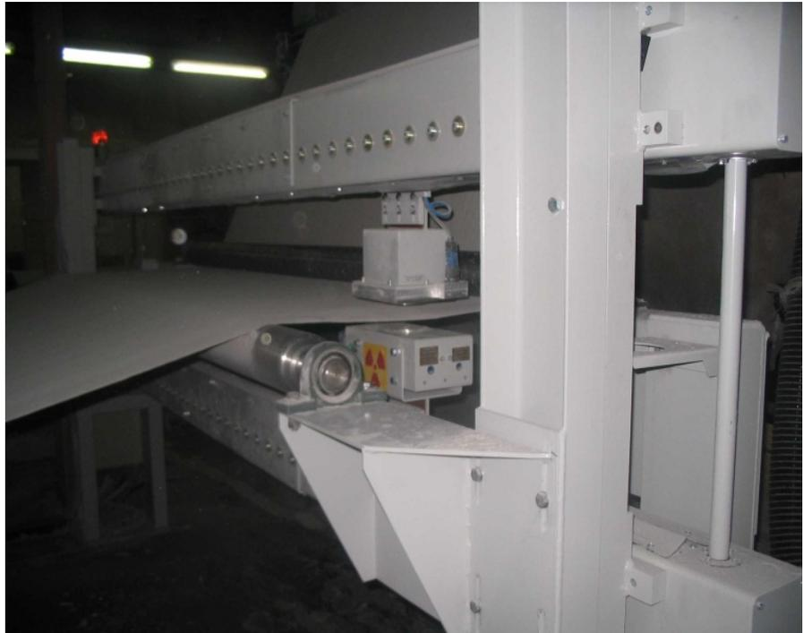
**Figure 21.** Traversing thickness gauge [25].
