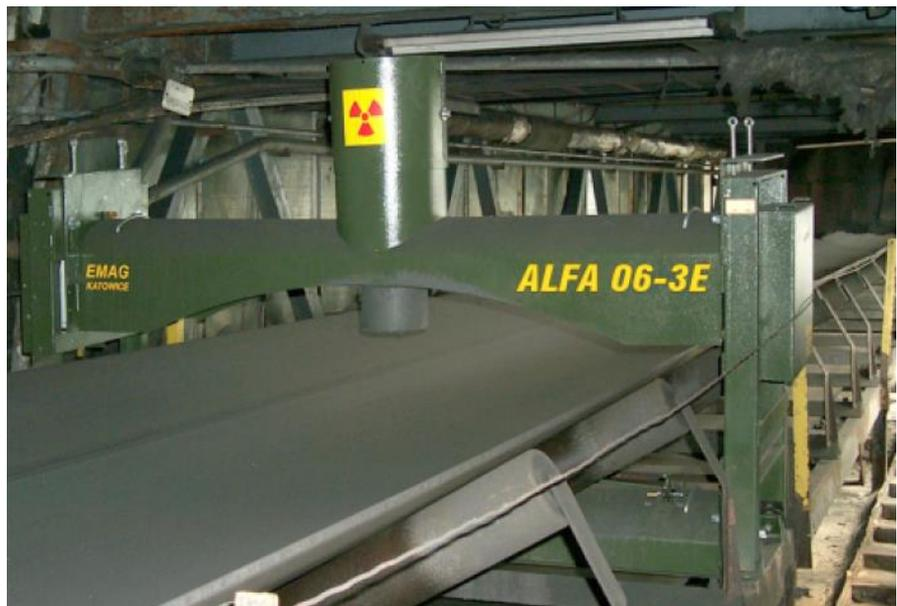
**Figure 7.** ALFA 06/3E at the coal processing plant Radiation source: <sup>137</sup>Cs (0.555 GBq) and <sup>241</sup>Am (11.1 GBq) [13].
