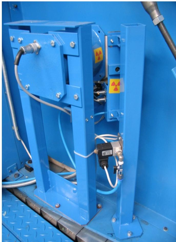
**Figure 22.** Backscattering densitometer for PE foam [25].
