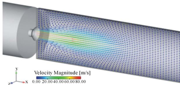
Figure 10. Steam velocity vector of size 10  $\mu\text{m}$ .
