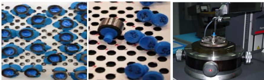
Figure 2. Resin curing process inside the holes (left). Samples for cylindricity measurement (center). Mahr Formtester MMQ 44 (right).
