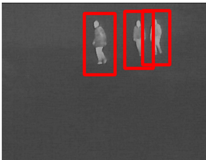
Figure 6. Human detection with thermal camera.
