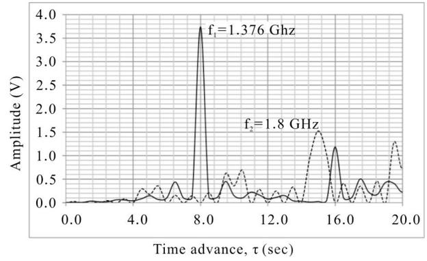
**Figure 3. Antenna array's response at typical S-PCN frequencies.**
