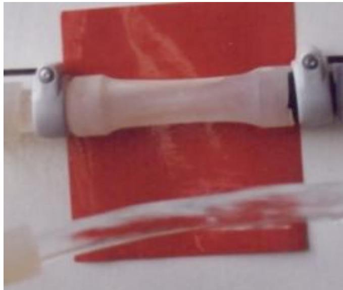
Figure 3. The chamber C around the G tube is made of soft rubber which is sucked in by the negative pressure gradient of the G tube. The interstitial pressure fluid has negative pressure of -7 ml water.
