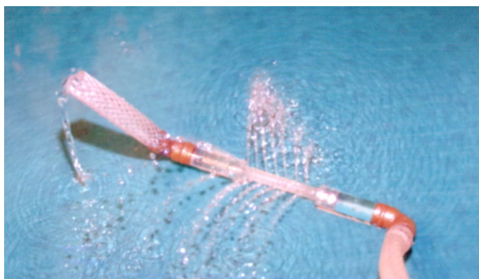
Figure 1. Shows the hydrodynamics of the porous orifice (G) tube. There is a pressure gradient at the wall of the G tube starting at the borifice with high suction and ending at exit with high filtration. The water comes out over the distal part and is sucked in over the proximal part of the G tube.
