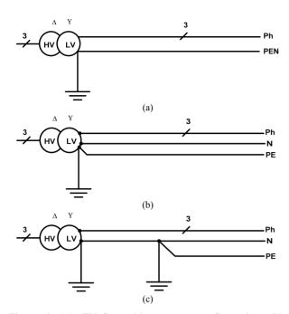
Figure 2. (a): TN-C earthing system configuration; (b): TN-S earthing system configuration; (c): TN-C-S earthing system.
