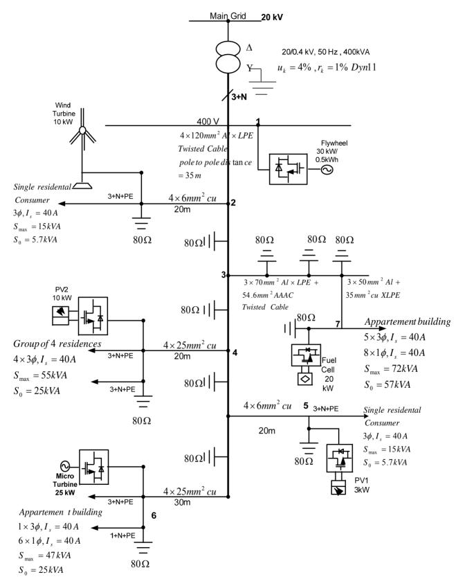
Figure 8. Single line diagram of the studied MG.
