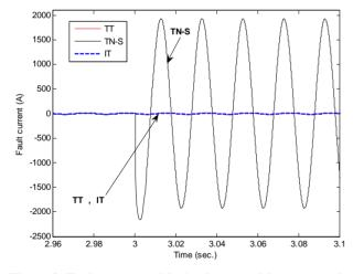
Figure 9. Fault current with the three earthing systems in the grid connecting mode.
