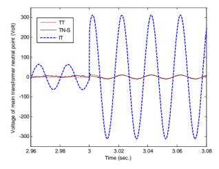
Figure 16. Main transformer neutral point's voltage.
