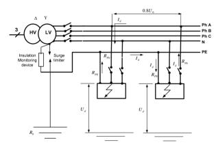
Figure 7. Second insulation fault current in IT system (distributed neutral).
