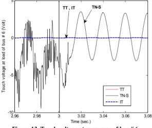
Figure 13. Touch voltage at consumer of bus # 6.
