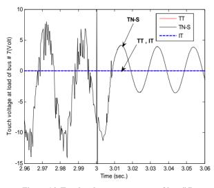
Figure 14. Touch voltage at consumer of bus # 7.
