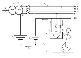
Figure 5. The fault behavior in the TT earthing system.
