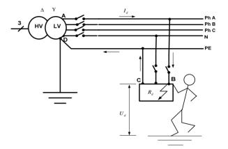
Figure 4. A fault behavior in the TN-S earthing system.
