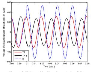
Figure 15. Voltage of healthy phases (at bus # 2).
