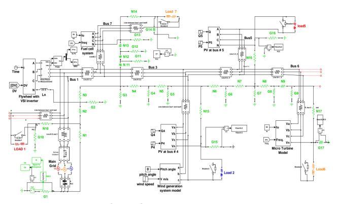
Figure 17. Matlab<sup>©</sup> /Simulink<sup>©</sup> Developed model for MG with the erathing system.
