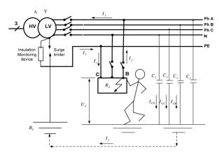
Figure 6. First insulation fault current in the IT earthing system.
