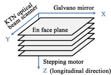
**Figure 2.** En face scanning for 3D-OCT data.
