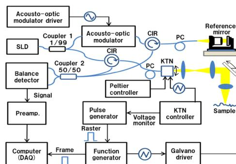
**Figure 1.** High-speed TD en face OCT system configuration. CIR: Circulator; PC: Polarization controller; DAQ: Data acquisition system.
