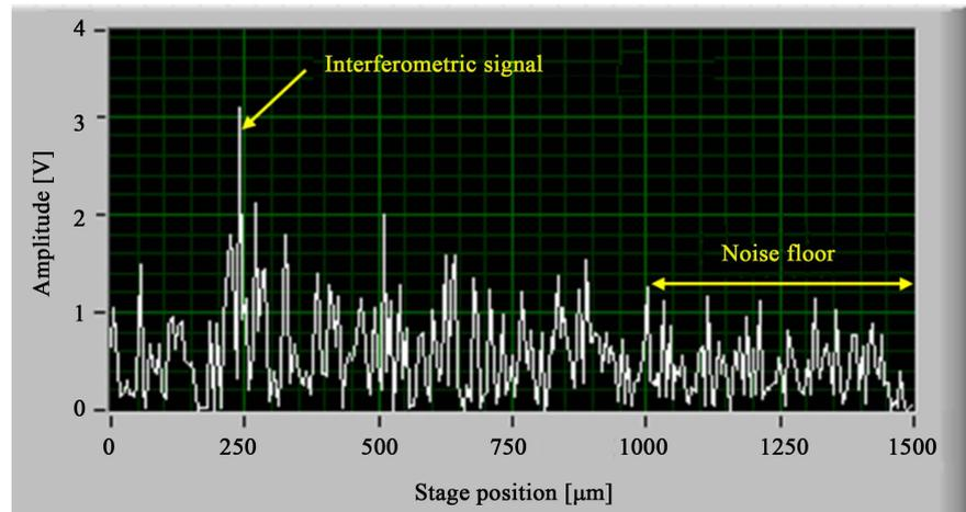
**Figure 5.** The measured signal-to-noise ratio (SNR) of the en face OCT system.
