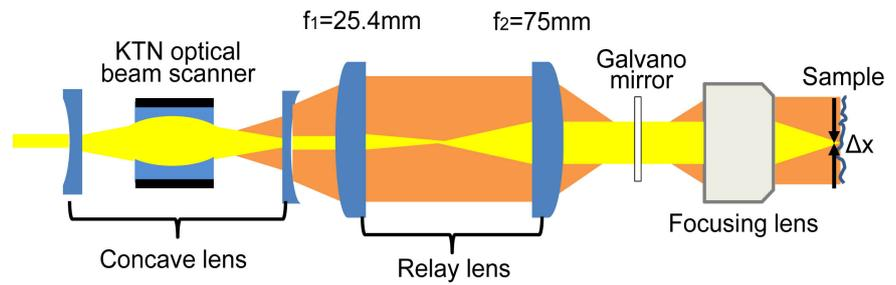
**Figure 3.** Beam propagation and optical arrangement of the sample arm.
