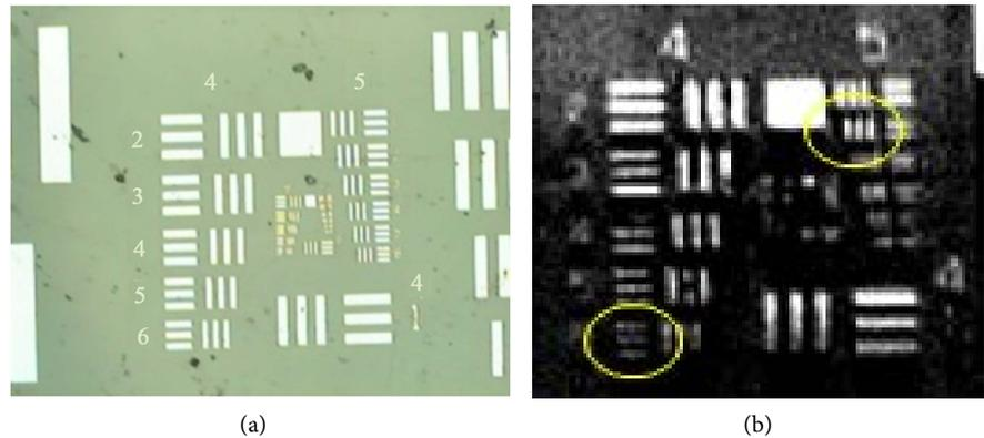
**Figure 4.** En face image of test chart (USAF 1951). (a) Photograph of test chart; (b) En face image of test chart.
