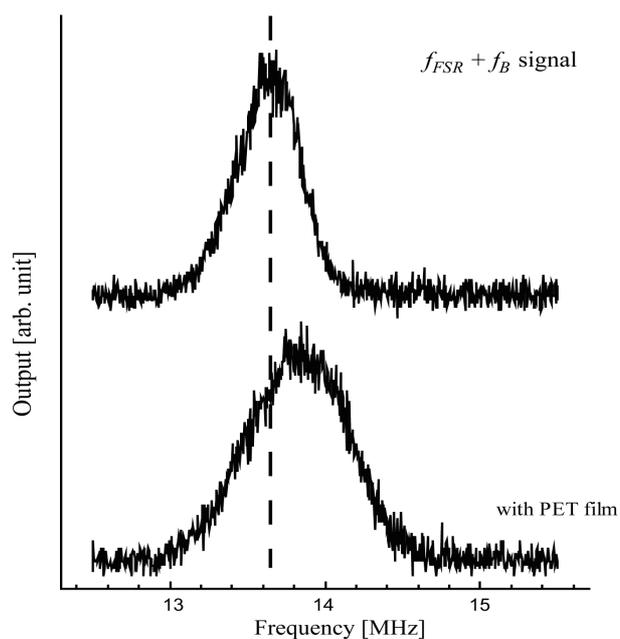
**Figure 5.** Power spectrum of  $f_{FSR} + f_B$  signal. The upper and the lower traces show without and with PET film.
