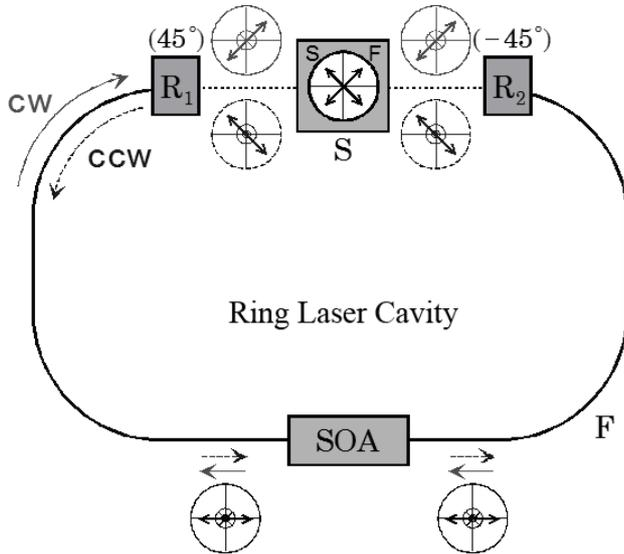
Figure 1. Schematic diagram of SOA-fiber ring laser.
