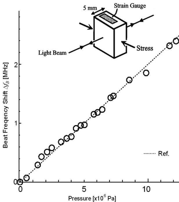
**Figure 6.** Beat frequency difference on applied pressure on fused silica.
