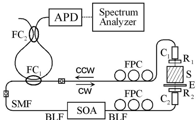
Figure 2. Configuration of SOA-fiber ring laser.
