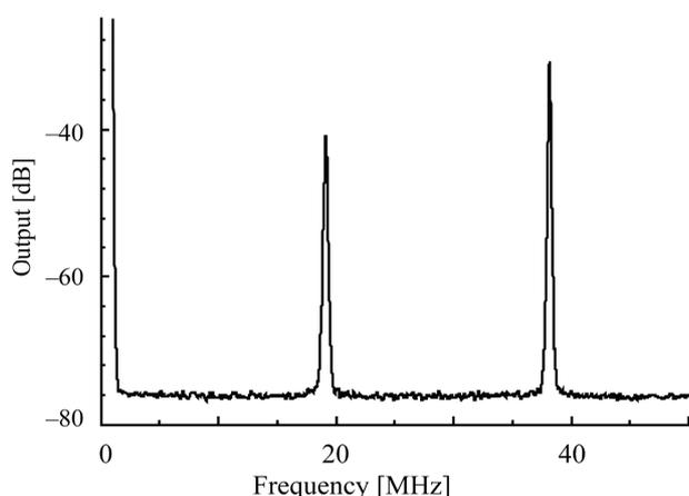
**Figure 3.** Power spectrum of SOA-fiber ring laser without birefringent media.
