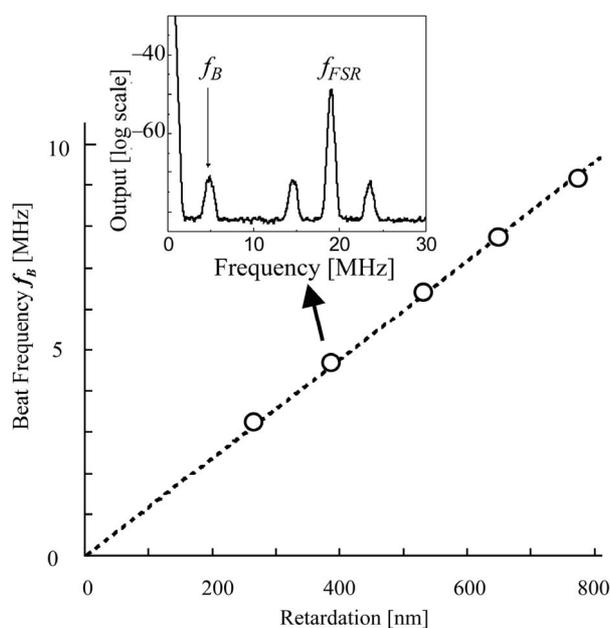
**Figure 4.** Change of frequency difference  $f_B$  with applied retardation. Inset power spectrum is the case of  $R = 387.5$  nm.
