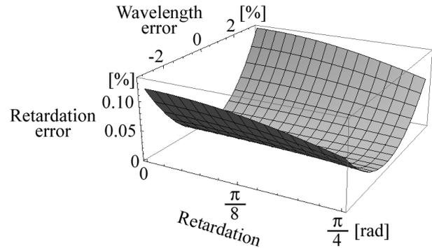
**Figure 7.** Retardation errors dependence on wavelength deviation.
