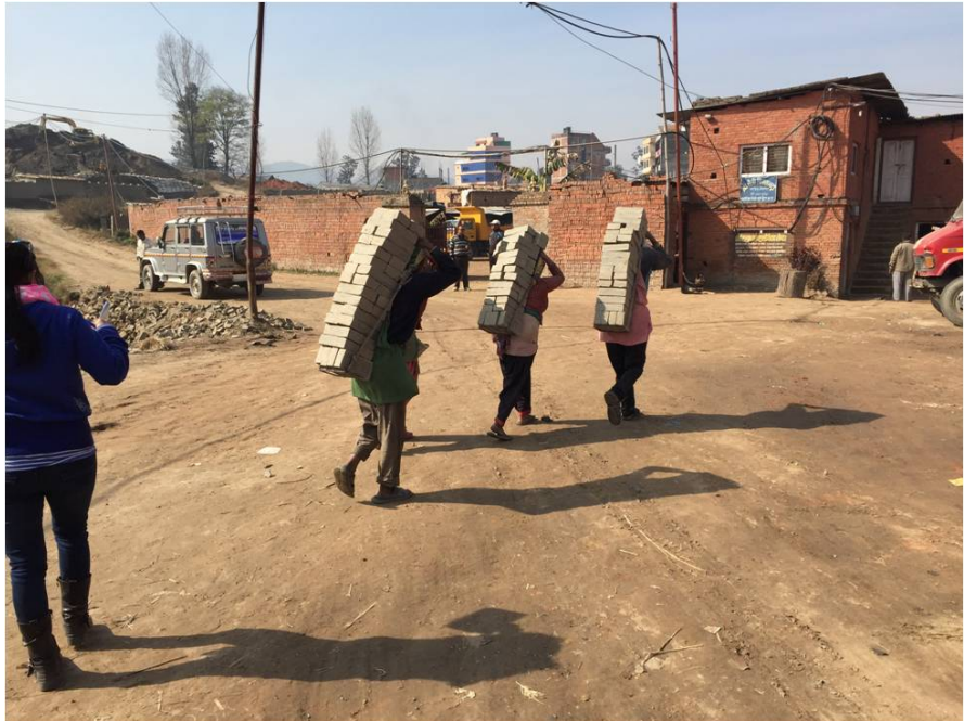
Figure 2. Workers carrying green bricks. Figure by Steven Thygerson.
