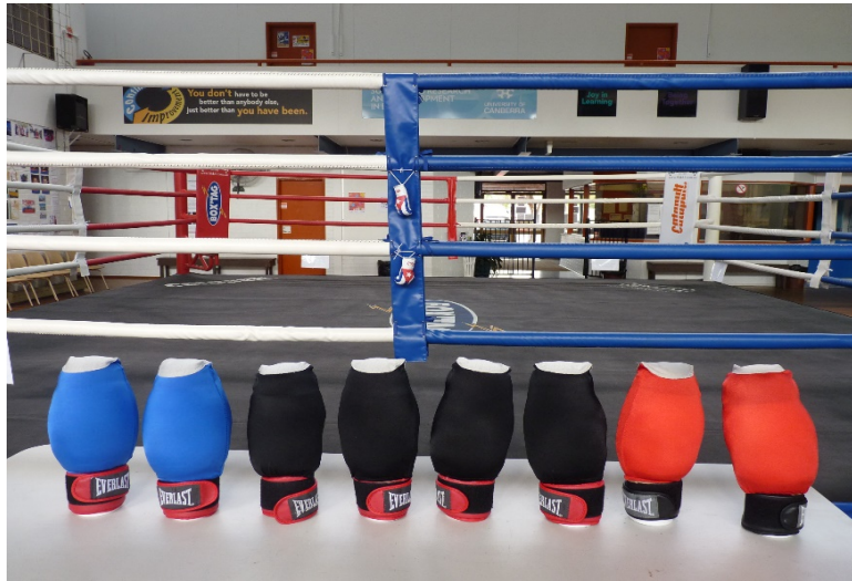
Figure 5. Prototype low-impact gloves with additional foam added to perimeter of glove to increase protection against impacts delivered with a part of the glove other than the bladder. The white areas at the top of the gloves are electrically conductive patches that formed part of automated scoring technology used in Box' Tag [50].
