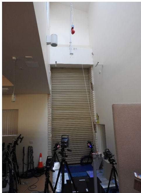
Figure 18. Drop testing system used for glove evaluation at the University of Canberra.
