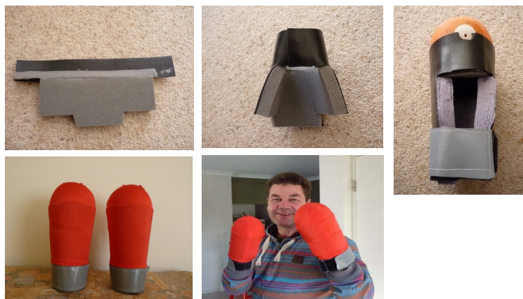
Figure 8. Overview of the construction of the first prototype low-impact gloves designed around the bladder.
