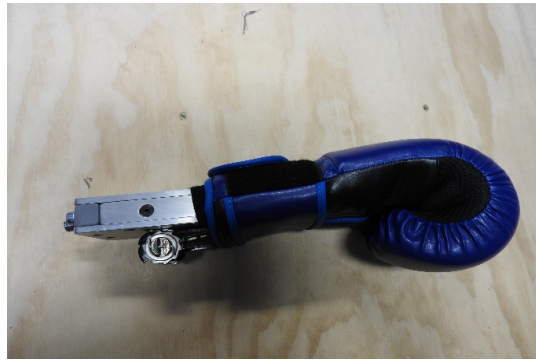
Figure 14. A conventional glove attached to the new mechanical fist, with the fist locked into the clenched position through use of a ratchet mechanism.
