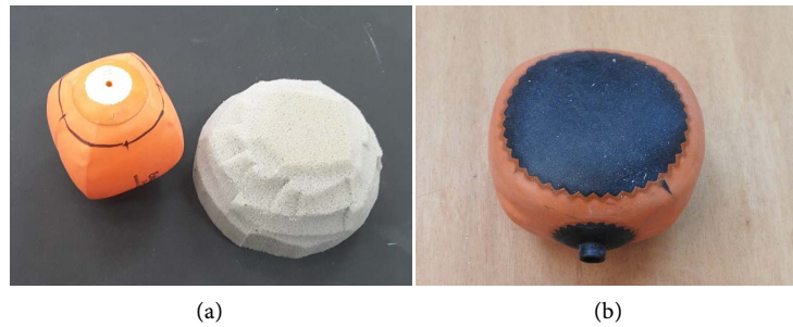
Figure 21. Construction of bladder for new prototype low-impact glove with capability for air release. The Size 1 soccer ball bladder in panel a was cut cross-sectionally at the point indicated by the black line. The foam skeleton was then inserted and the unit was sealed with a truck tyre patch (panel b). A port allowing air release and reuptake was then added.
