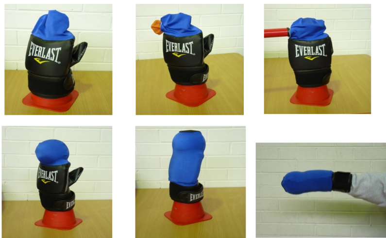
Figure 4. Construction of highly deformable prototype gloves. The end-section of a standard training glove was cut off and replaced by a sewn-on, stretchable lycra bag with a sealable opening for insertion of a small spherical bladder, which could then be inflated. A second lycra bag could subsequently be pulled over the whole complex to provide shape and stability and to enclose the thumb. A glove with fist in position behind the bladder is shown on the bottom right.
