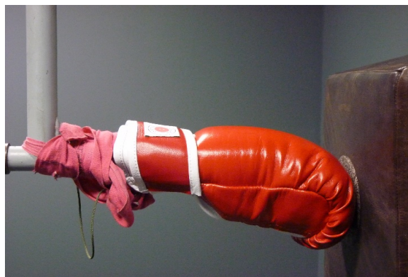
Figure 13. First tests involving use of a pendulum apparatus with attached mechanical fist for glove testing. The photograph shows a prototype low-impact glove contacting the pad covering the wall-mounted force plate.
