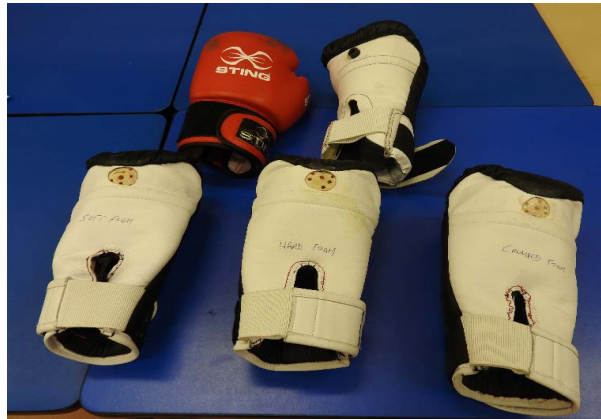
Figure 26. Gloves used in testing the effects of a new pattern of air openings and variation in foam characteristics of the bladder skeleton on the impact damping performance of ARLI gloves.
