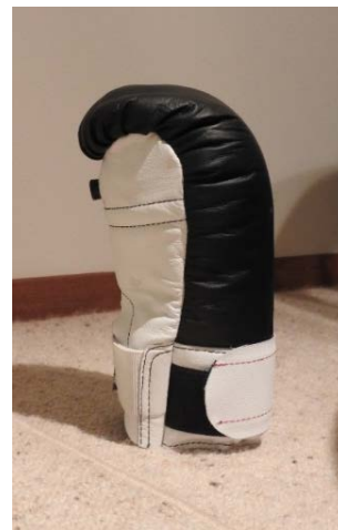
Figure 22. Prototype low-impact glove allowing movement of air between glove bladder and external environment. The port for air exchange can be seen on the front surface of the glove.
