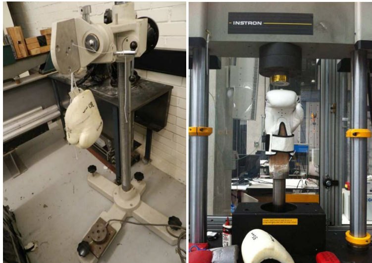
Figure 2. Equipment set-up for drop-weight and INSTRON testing of prototype gloves and air-filled foam materials.
