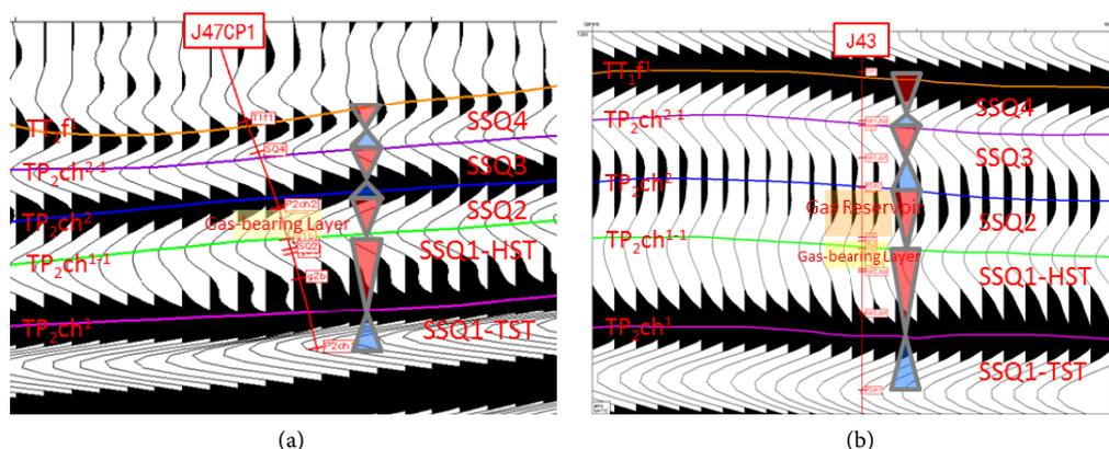
**Figure 6.** Seismic responding features of Bioclastic shoal in Changxing Formation, Jiannan area (Well J47CP1 and Well J43).
