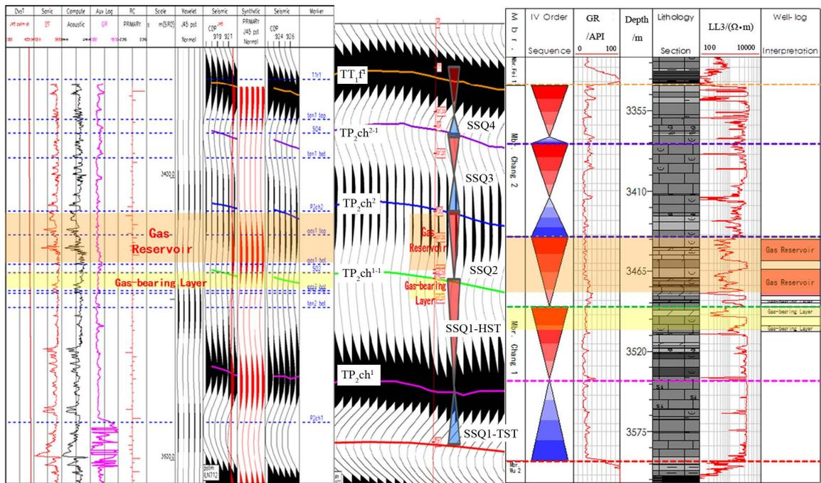
Figure 5. Synthetic seismic record of Changxing Formation in Well J45.
