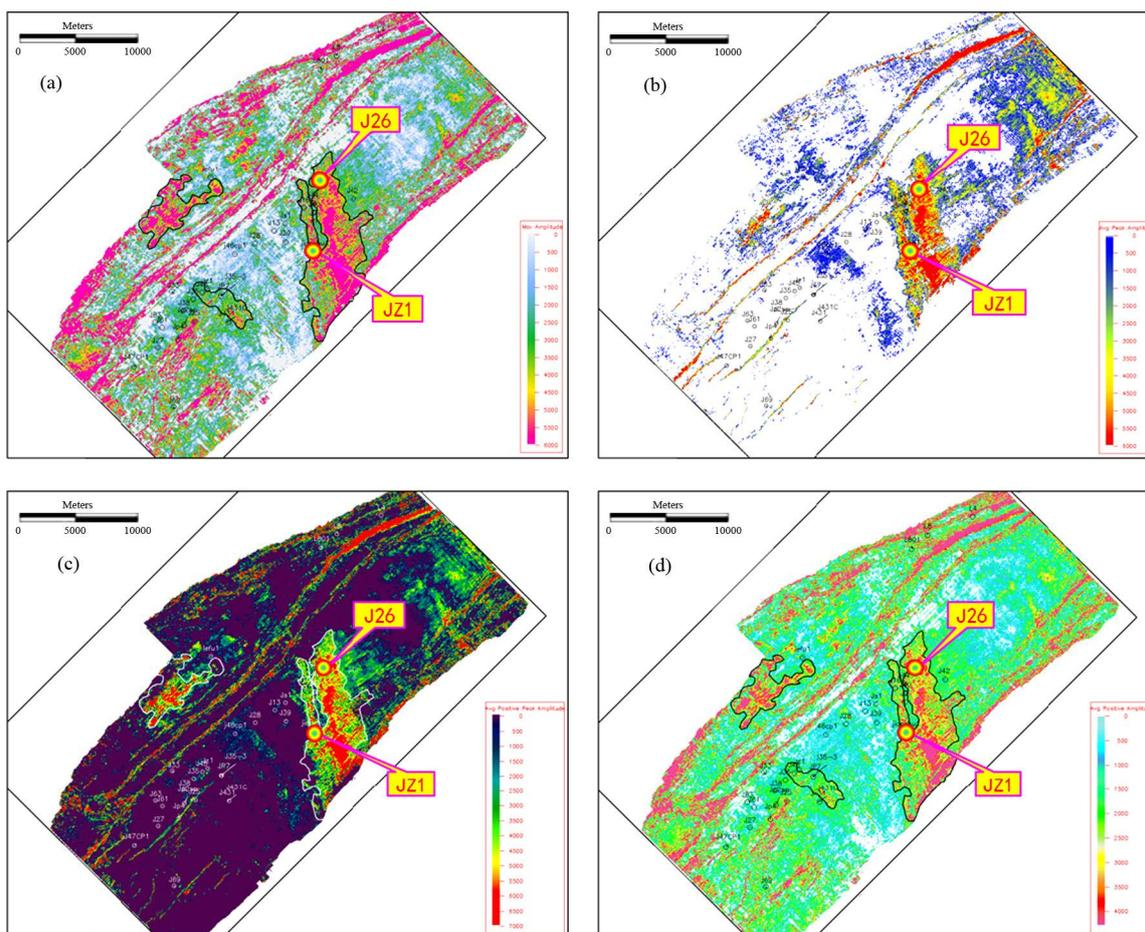
**Figure 7.** Seismic attribute map of SSQ1-HST, Changxing Formation, Jiannan area. ((a) Maximum amplitude; (b) Average peak amplitude; (c) Average peak value; (d) Average positive amplitude).
