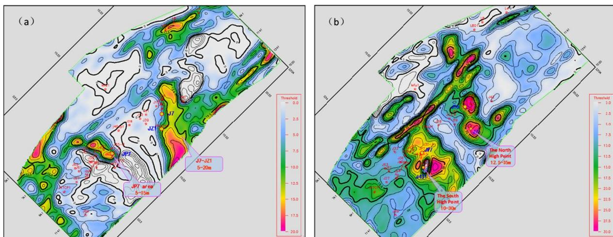
**Figure 9.** The reservoir thickness prediction map of Changxing Formation in Jiannan area. ((a) SSQ1 reservoir thickness, (b) SSQ2 reservoir thickness).
