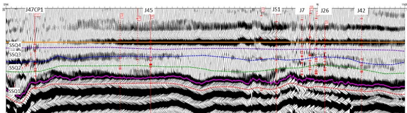
Figure 4. Seismic section from J47CP1 to J42 of sequence classification in Jiannan area.
