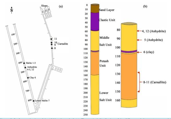
**Figure 5.** Surface projection of the 1200 m long shaft (a). The vertical distribution of the different salt layers (core sample) at the right in the diagram. Modified after URL: <u>http://www.apmcnet.com/en/project\_bamnet.php</u> (query 20.09.2013).
