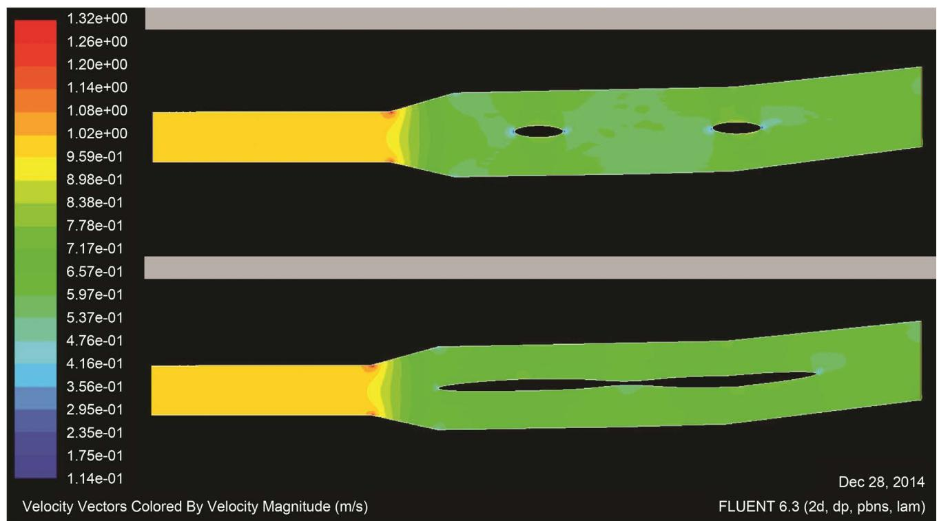
**Figure 9.** Velocity, top: initial domain DOM0, bottom: modified domain DOM3. (Less flow instabilities in the middle region).
