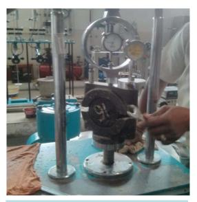
Figure 9. Performing marshal stability test.
