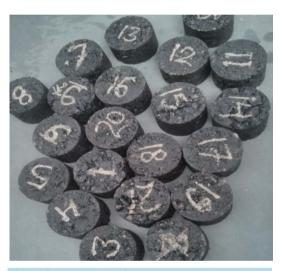
Figure 8. Prepared specimens.
