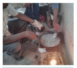
Figure 4. Adding shredded plastic to aggregates.
