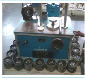
Figure 7. Marking of prepared moulds.
