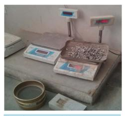
Figure 2. Aggregate weighing.
