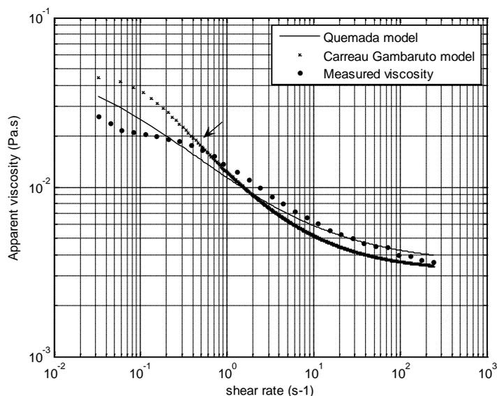
**Figure 1.** Comparison between measured viscosity [6], Carreau-Gambaruto-model and Quemada model. The arrow shows the inflection point on the viscosity curve.
