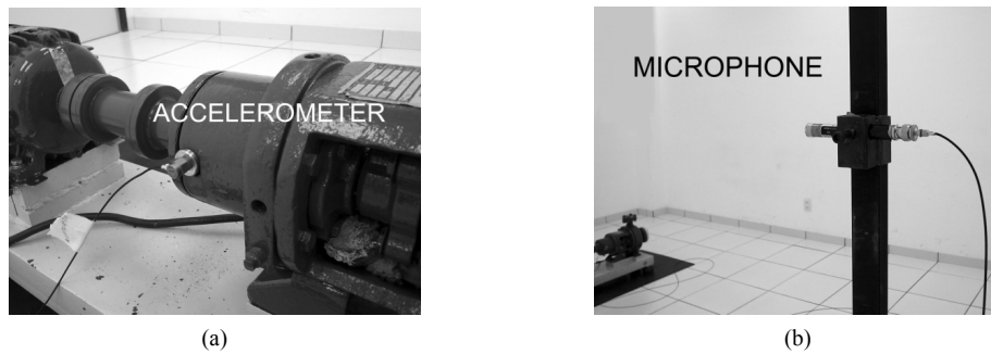
Figure 2. Experimental apparatus: (a) System input, primary source sensor: pump accelerometer (100mV/g) signal; (b) System output, passive sensor: microphone (50mV/Pa) signal.
