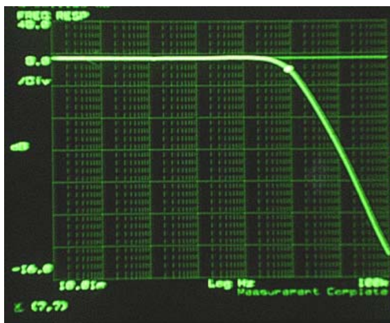
Figure 9. Measured transfer function of the INA.
