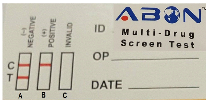
Figure 1. Interpretation of urine screening test: (A) negative, (B) positive, and (C) invalid test.
