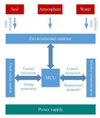
Figure 2. Hardware system structure diagram.
