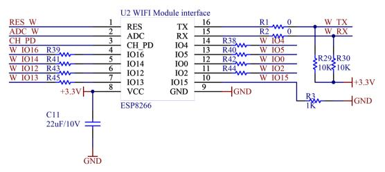
Figure 3. Wireless module circuit diagram.
