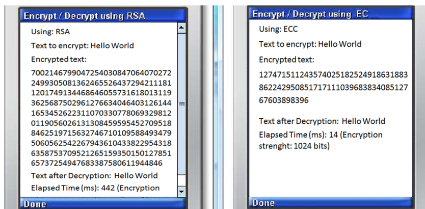
Figure 3. Encrypt/Decrypt using RSA and ECC for comparison.
