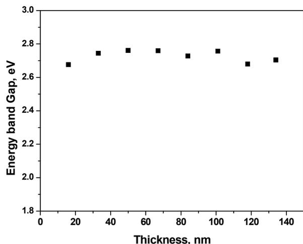
Figure 4. Energy band gap for different thickness of Alq<sub>3</sub>.
