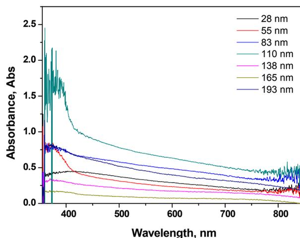
**Figure 3.** The optical absorption of NPB measured at different thicknesses.
