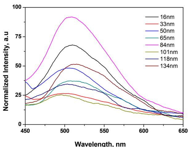
Figure 6. The PL performance with the different thickness of Alq<sub>3</sub>.
