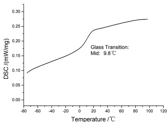
**Figure 1.** DSC curve of Styrene-acrylic latex (BA:MMA:St = 33:19:18).
