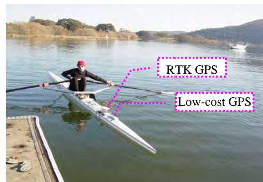
Fig. 12. RTK geodetic (carrier phase) and low-cost (code-only) GPS receivers mounted on the same boat
