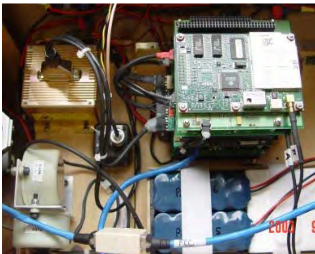
Fig. 6. Flight control system with IMU (top left), tilt sensor (bottom left), GPS (top right) and vision camera (centre).
