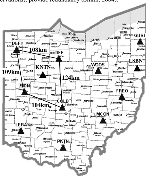
Fig. 3a The CORS subnetwork used in the experiments.
