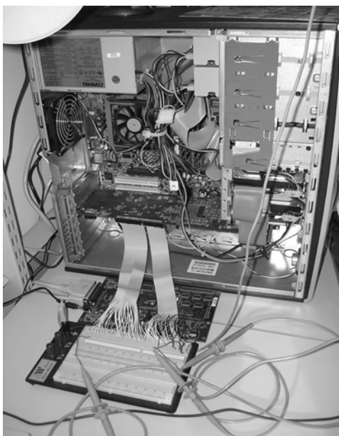
Fig. 2 SDR platform for the Navigation Unit implementation.
