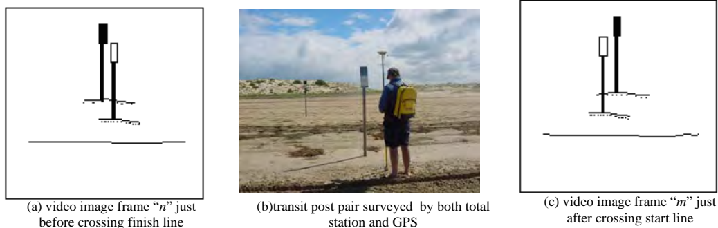
Fig. 3 Diagrammatic view of the transit posts surveyed by both conventional and GPS methods (b) and video image frames “m” and “n” at the start (c) and finish (a)
