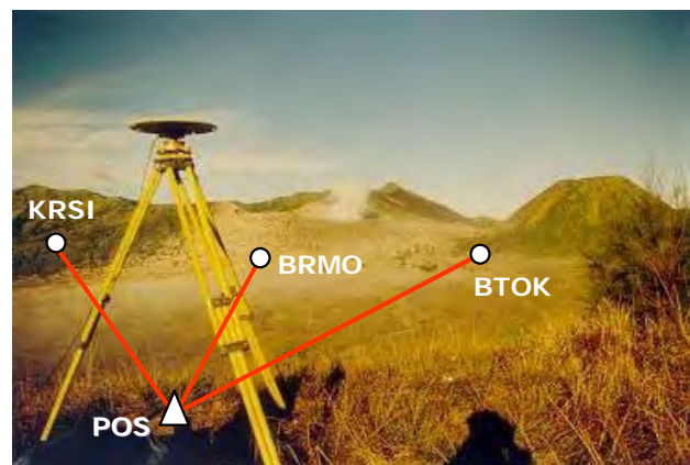
Fig. 4 EDM monitoring network in Bromo.
