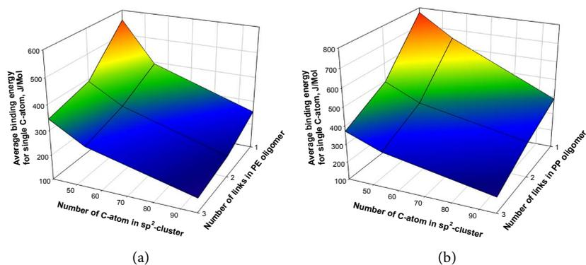
**Figure 5.** The dependence of average binding energy attributable to one atom of nanocomposite with various  $sp^2$ -cluster of CNT and PE (a) and PP (b) oligomer fragments.
