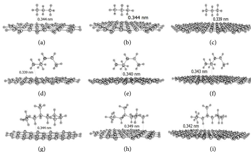
**Figure 4.** The structure of different length PP fragments in intermolecular complexes with graphene-like clusters of different sizes, which simulate a fragment of the outer surface of CNT.
