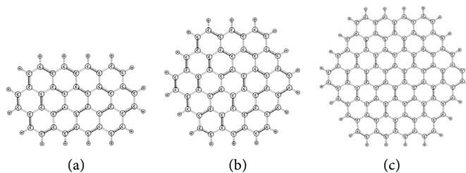
**Figure 1.** Models for the fragment of the outer surface of CNT by the general composition: (a)  $C_{40}H_{16}$ ; (b)  $C_{54}H_{18}$ ; (c)  $C_{96}H_{24}$ .
