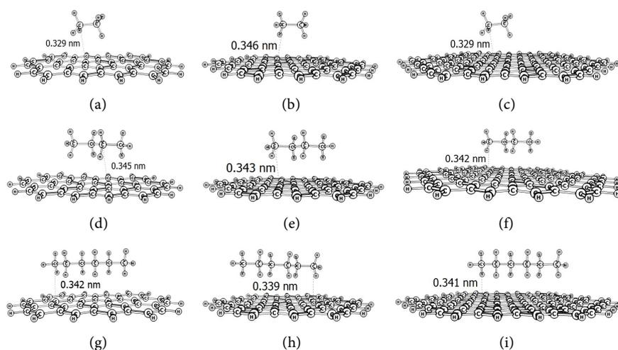
**Figure 3.** The structure of different length of PE fragments in intermolecular complexes with graphene-like clusters of different sizes, modeling a fragment of the outer surface of CNT.
