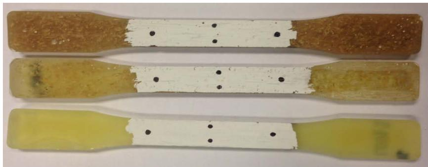
**Figure 6.** 0%, 10% and 30% RHP samples with gage markers.
