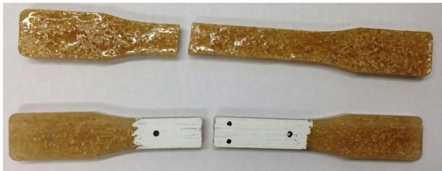
**Figure 5.** RHP-Epoxy 0.30 Volume Fraction Samples—Premilled (Top) and Milled (Bottom).
