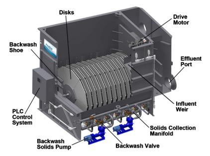
**Figure 4.** A typical disc filter unit found in the market for final separation of solids (Source: Aqua Aerobic Systems, Inc. Rockford, US).
