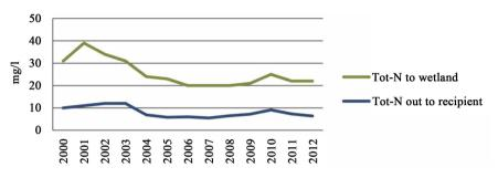
**Figure 7.** Inlet and outlet nitrogen concentrations to the wetland stage at the Nynäshamn WWTP.
