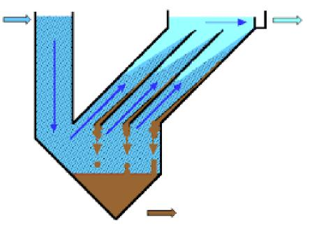
Figure 1. A typical lamella sedimentation function model (source: Nordic Water Products).
