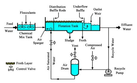
Figure 2. A typical flow scheme for wastewater based on dissolved air flotation.
