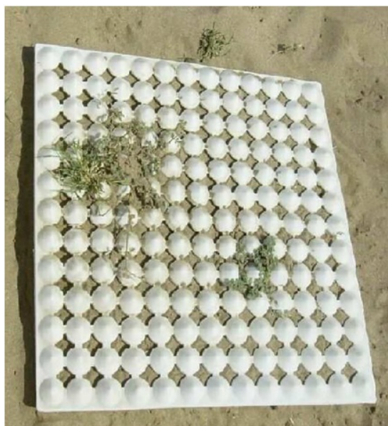
Figure 2. Reflective carpet capturing vapour up-flux and turning the desert green in 5 months.
