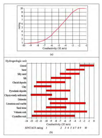
Figure 8. *Hydraulic conductivity* (a) values and ratings and (b) ranges of the main hydrogeological units, values and ratings assigned by the SINTACS method (according to [5], modified).
