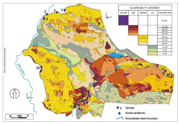
Figure 4. Matese Mts. Aquifer pollution vulnerability map computed using the SINTACS method (from [10]).
