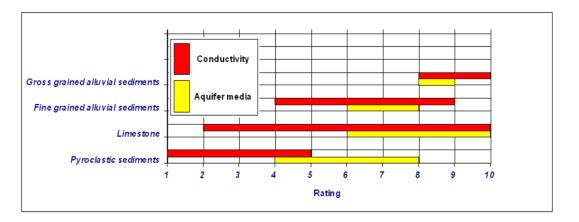
Figure 9. *Hydraulic conductivity* and *Aquifer media* ranges of the hydrogeological units present in the sample areas and ratings assigned by the SINTACS method.
