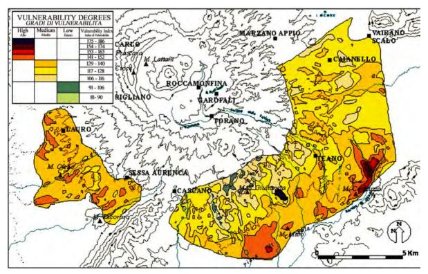
Figure 5. Roccamonfina Volcano Aquifer pollution vulnerability map computed using the SINTACS method (according to [7]).
