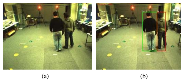
Figure 13. An example of tracking occluded objects in one depth layer. (a) Input frame (having occlusion objects); (b) Output (tracking occlusion objects in different layers).
