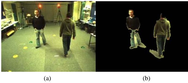
Figure 3. Foreground segmentation. (a) input image; (b) segmented foreground image.
