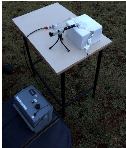
Figure 2. The experimental setup performed in the field (outdoor) with 120 m laser beam length. It is shown the high voltage power supply (grey box) where the PZT4 ceramic disc supported on the styrofoam box is connected by strips of aluminum. The laser pointer is supported by a tripod and it is activated continuously.
