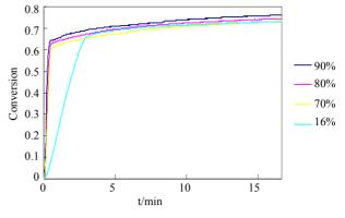
Figure 8. Conversion rate of CaO carbonation at different concentration of  $CO_2$  (700<sup>•</sup>C).
