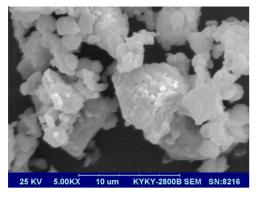
Figure 2. Porous calcined limestone particle.
