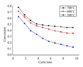
Figure 11. Multiple cycle calcinations/carbonation reaction.
