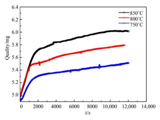
Figure 13. Direct desulfurization TG curve.
