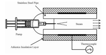
Figure 6. Single channel syringe infusion pump and pipe heating system.
