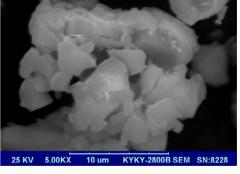
Figure 1. Unreacted limestone particle.
