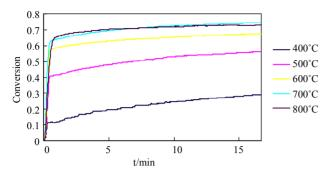
Figure 7. Conversion rate of CaO carbonation at different temperatures.
