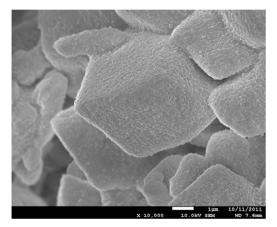
Figure 16. Indirect desulfurization particle surface morphology.
