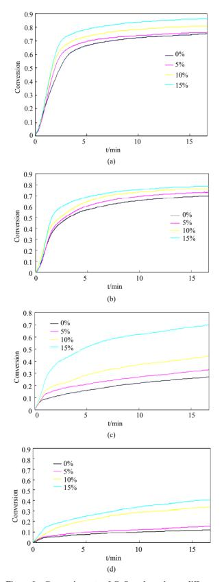
Figure 9. Conversion rate of CaO carbonation at different concentration of  $H_2O$ . (a) 700°C; (b) 600°C; (c) 500°C; (d) 400°C.
