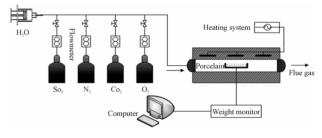
Figure 5. Tube furnace heating system.
