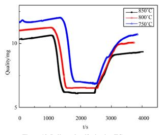
Figure 12. Indirect desulfurization TG curve.
