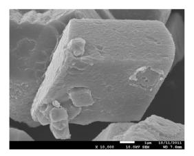
Figure 17. Direct desulfurization particle surface morphology.
