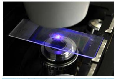
Figure 2. Blue light of a laser beam cutting a specific region, or cells of interest from a biological tissue laid after treatment on a microscope slide.
