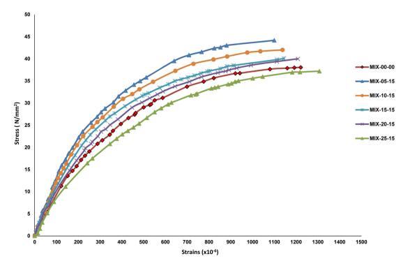
**Figure 4.** Stress-strain curves of mixtures contained cement kiln dust (CKD) 5%, 10%, 15%, 20% and 25% with constant 15% silica fume (SF), compared with control mixture 0% CKD with 0% SF after 28 days.
