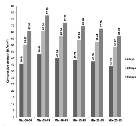
**Figure 1.** Compressive strength of mixtures contained cement kiln dust (CKD) 5%, 10%, 15%, 20% and 25% with constant 15% silica fume(SF), compared with control mixture 0% CKD with 0% SF After 7, 28 and 56 days.
