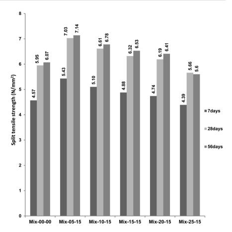
**Figure 2.** Split tensile strength of mixtures contained cement kiln dust (CKD) 5%, 10%, 15%, 20% and 25% with constant 15% silica fume(SF), compared with control mixture 0% CKD with 0% SF After 7, 28 and 56 days.
