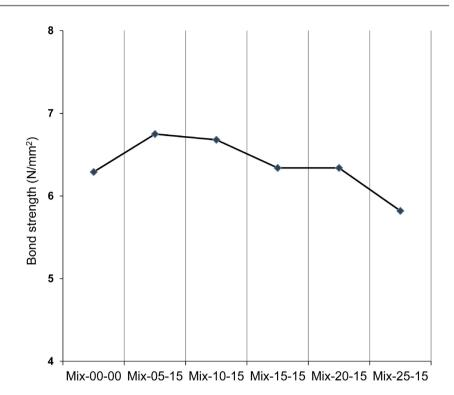
**Figure 5.** Bond strength of mixtures contained cement kiln dust (CKD) 5%, 10%, 15%, 20% and 25% with constant 15% silica fume(SF), compared with control mixture 0% CKD with 0% SF after 28 days.
