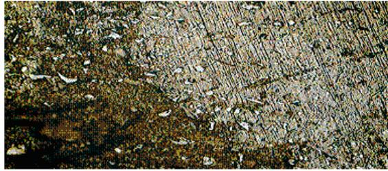
Micrograph 3: Tin tailings with (10% Al-Si alloy). x200 microstructure contains  $\text{SiAl}_6$  (white) and the ceramic phase (black) (200x).
