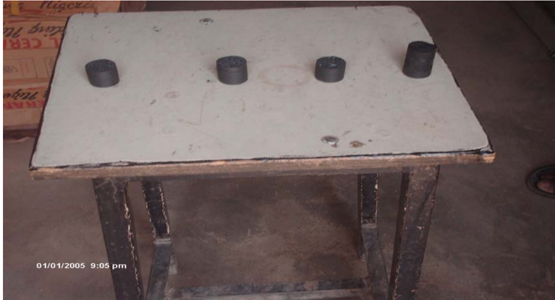
Plate 3: Photograph of the moulded Bagasse ash after firing
