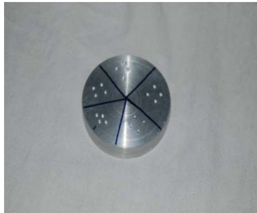
Fig. 4. Pictorial view of sample for comparing indentation load with normalized displacement.
