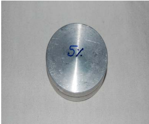
Fig. 2. Pictorial view of sample containing 5% SiC by weight for hardness test Fig. 3. Pictorial view of samples for impact test
