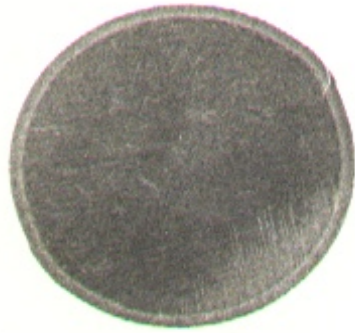
Plate 1(a) Macrostructure of a specimen, carburized at 940 0 C for 3 hours The carburizer contained 20% Na 2 CO 3 Etched in 25% Nital. Magnification : x 2
