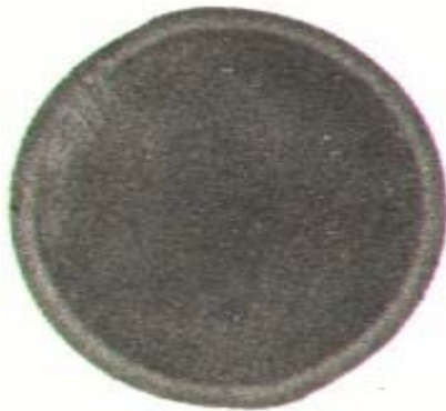
Plate 2 (a) Macrostructure of a specimen, carburized at 900 0 C for 3 hours The carburizer contained 20% Na 2 CO 3 Etched in 25% Nital. Magnification: x2
