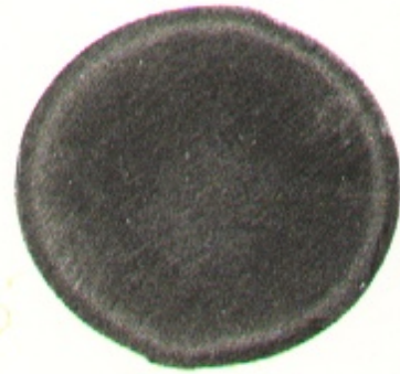
Plate 1(b) Macrostructure of a specimen, carburized at 940 0 C for 4 hours The carburizer contained 20% Na 2 CO 3 Etched in 25% Nital. x2 Magnification : x2
