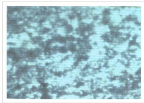
Plate11. 70% Deformation, 450°C, 30min
