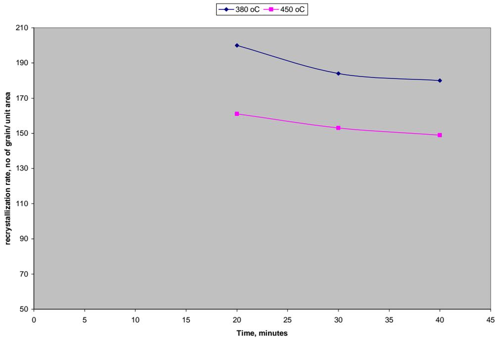
Figure 4. Effect of holding time on recrystallization rate at constant %cold deformation (90%).
