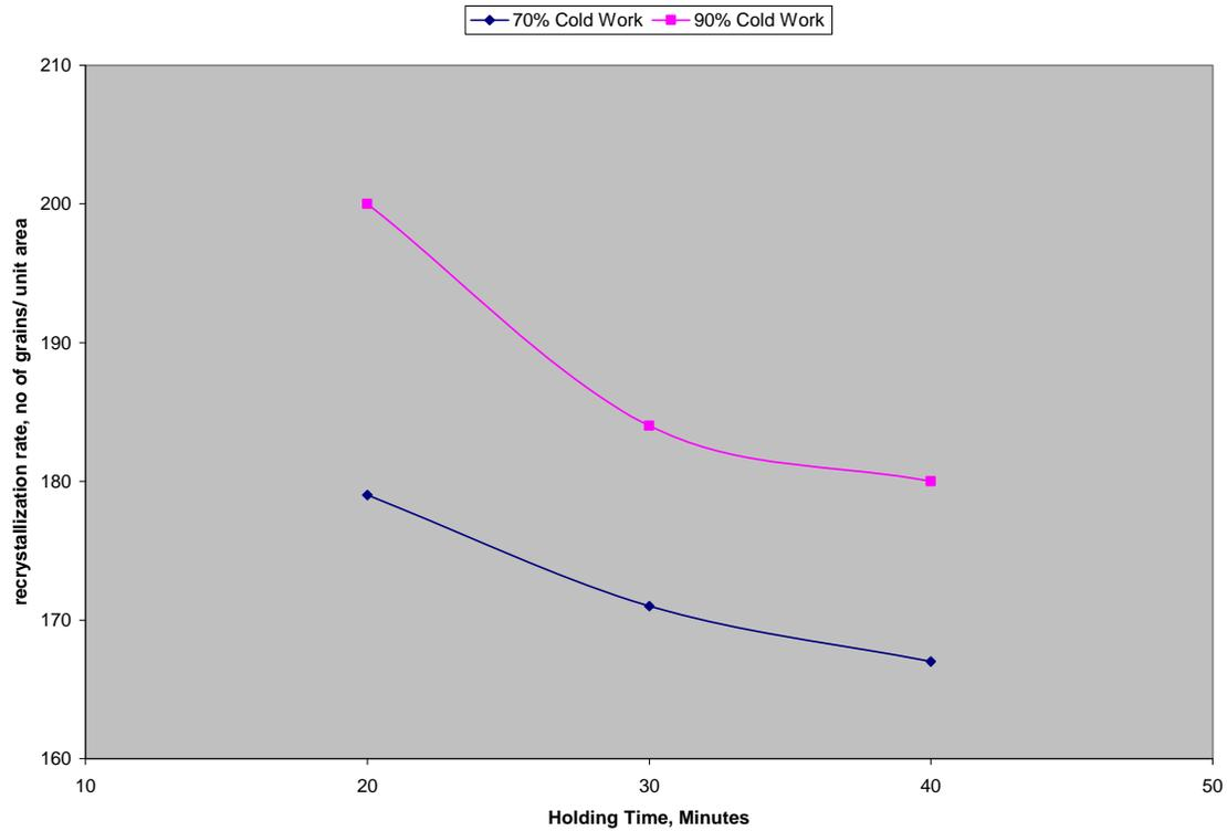
Figure 1. Effect of holding time on recrystallization rate at constant temperature ( $380^{\circ}\text{C}$ ).
