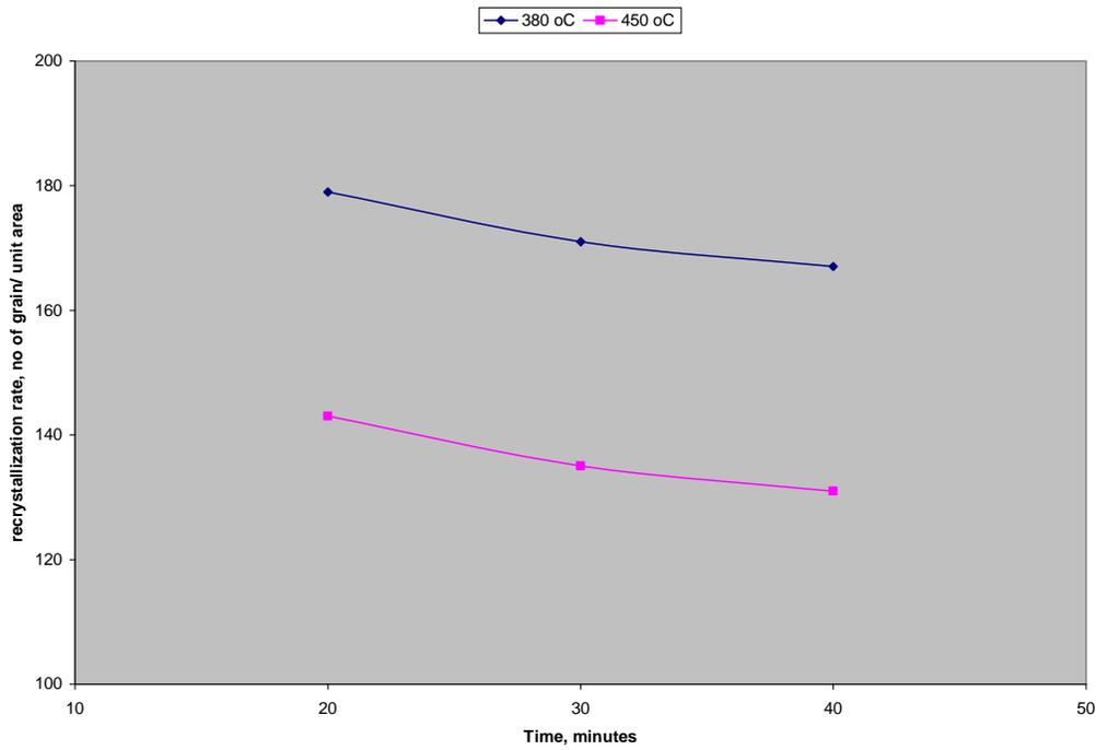
Figure 3. Effect of holding time on recrystallization rate at constant %cold deformation (70%)
