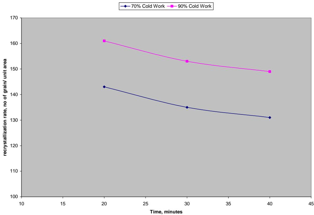
Figure 2. Effect of holding time on recrystallization rate at constant temperature ( $450^{\circ}\text{C}$ ).
