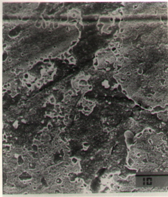
Fig.5. Scanning electron micrograph of a corroded AISI 321 SS after 20 days of exposure x 5000
