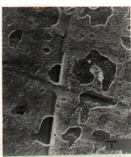
Fig.4. Scanning electron micrograph of a corroded AISI 304 SS after 20 days of exposure x 1000
