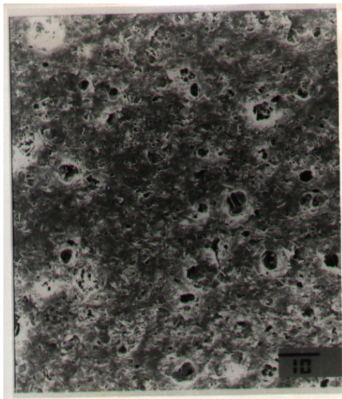
Fig.2 Scanning electron micrograph of a corroded AISI 430 SS after 20 days of exposure x 1000
