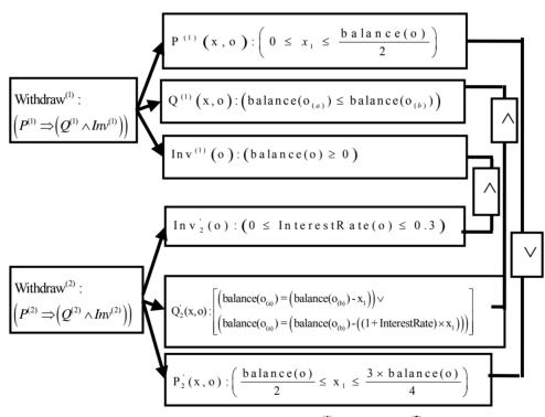
Figure 8. Constraints of withdraw<sup>(1)</sup> and withdraw<sup>(2)</sup>.
