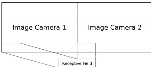
**Figure 1. Forming a receptive field of a node in the bottom layer in the stereoscopic setup-example**
