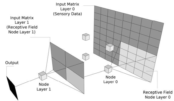
**Figure 2. Example, two layer hierarchy of nodes in one time step. Layer 1 contains a single node therefore input matrix of the Layer 1 and receptive field of the node in Layer 1 are identical**
