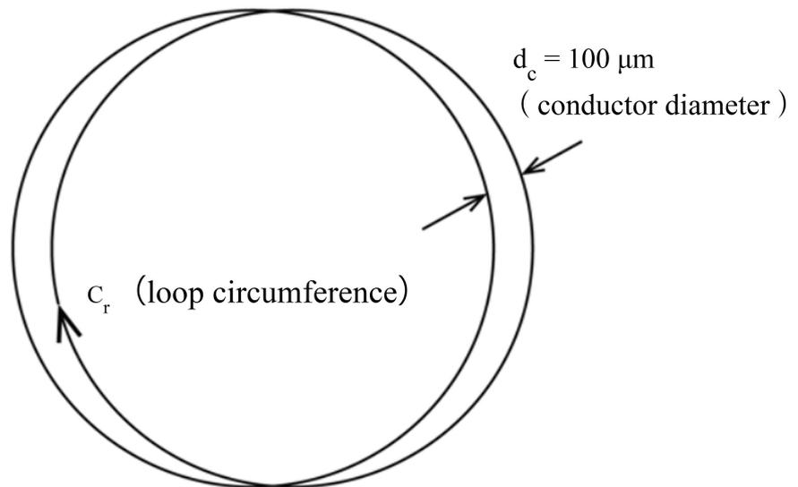
**Figure A-3.** Application area of Lorentz force for a single conductor loop in an SMES torus.
