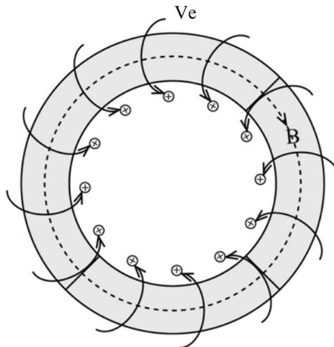
**Figure A-2.** Magnetic field in an SMES torus core.
