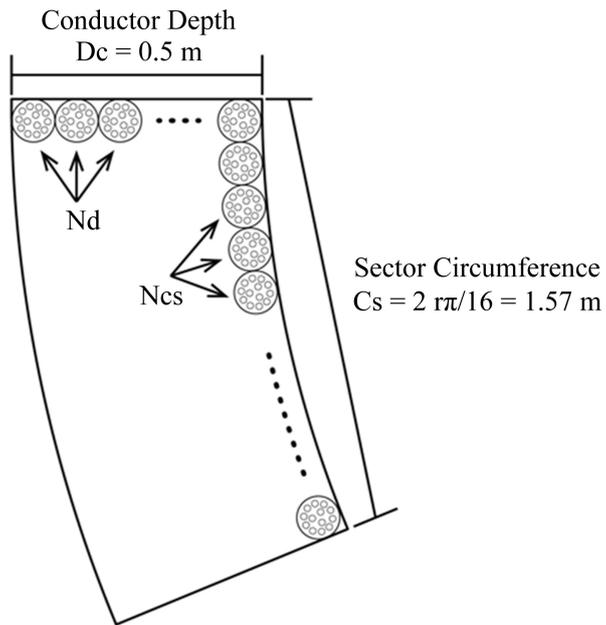
**Figure 7.** Conductor packing in each sector.
