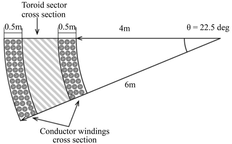
**Figure 6.** Conductor cross section in each sector.
