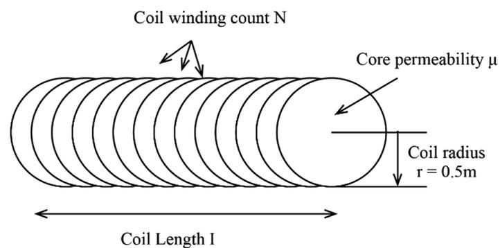
**Figure 8.** Geometry determining inductance.
