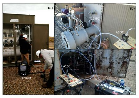
**Figure 2.** Examples of HVS and installed MFM measurements (a) HVS of Fisher<sup>™</sup> 4660 CPC with HHP exhaust check; (b) Alicat MFM installed on exhaust port of Kimray T12 IPC; (c) supply line measurement of two WellMark 6900 IPCs with Alicat and Fox MFMs in series (right), and a Fisher<sup>™</sup> 4660 CPC with an Alicat MFM (left).
