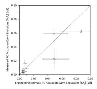
Figure 5. Comparison of EEE (EAe) and measured actuation events (MAe). Error bars for *EAe* (high/low) represent  $\pm 20\%$  actuation volume,  $\pm 20\%$  pressure, and -/+20% temperature based on conditions at the time of the survey. Error bars for MAe are minimum and maximum measured values.
