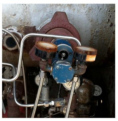
Figure 3. An older WellMark 6900 IPC found to be malfunctioning.
