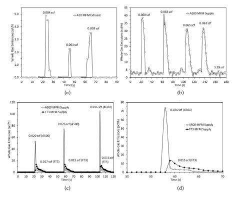
**Figure 4.** Manual actuation experiment of (a) Kimray T12 tank burner IPC; (b) complex Kimray T12 Separator IPC with malfunction; (c) Wellmark 6900 dump valve with both Alicat and Fox MFMs; and (d) Expanded view of (c).
