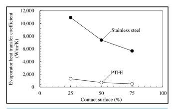
**Figure 6.** Effect of contact area on evaporator heat-transfer coefficients for PTFE and stainless steel wicks.
