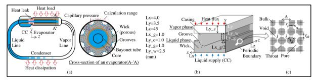
Figure 1. (a) Schematic of a loop heat pipe, (b) computational domain, and (c) representation of pore network model for fluid analysis in the wick.
