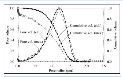
**Figure 3.** Comparison of the measured and calculated pore radius distributions. Vertical axes are normalized by the maximum value.
