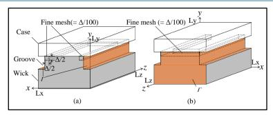
**Figure 2.** Liquid-vapor interface ( $\Gamma$  interface, orange area) and region of fine mesh (volime in dotted line). (a) front view and (b) rear view.
