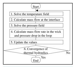
Figure 4. Flow chart of the numerical algorithm.
