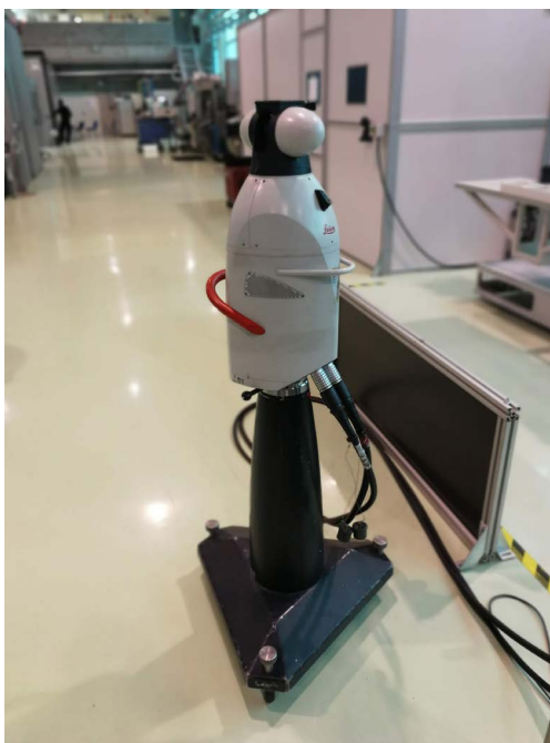
Figure 3. The laser tracker measures distances with a micrometric accuracy. It serves as as ground truth to measure localization errors.
