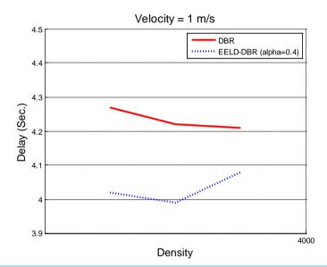
Figure 6. Delay comparison between DBR and EELD-DBR, delay results are in second unit, network density has variations from 1000 to 3000 nodes and also velocity (mobility of all nodes) is 1 m/s (fixed). This figure clearly illutrates lower delay of EELD-DBR than DBR.
