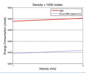
Figure 3. Consumed energy between DBR and EELD-DBR, consumed energy results are in joule unit, network density is fixed and equal to 1000 nodes and also velocity (mobility of all nodes) is selected between 1 and 5 m/s.
