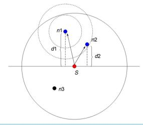
Figure 1. Showing the DBR routing protocol, DBR selects suitable nodes to cooperate in routing<sup>1</sup>.
