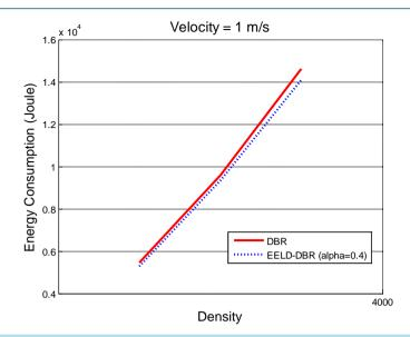
Figure 5. Consumed energy between DBR and EELD-DBR, consumed energy results are in joule unit, network density has variations from 1000 to 3000 nodes and also velocity (mobility of all nodes) is 1 m/s (fixed).
