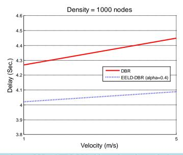
Figure 4. Delay comparison between DBR and EELD-DBR, delay results are in second unit, network density is fixed and equal to 1000 nodes and also velocity (mobility of all nodes) is selected between 1 and 5 m/s.
